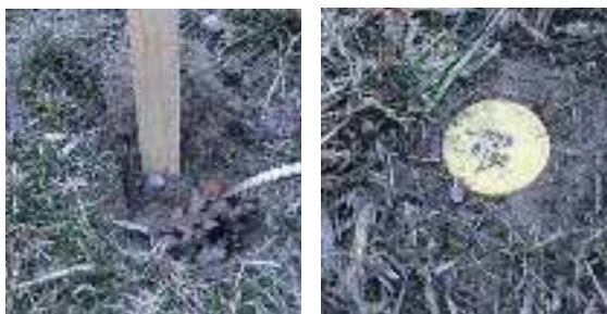
Property boundary pins, driven into the ground by a licensed surveyor, mark the boundary corners of a homeowner’s property. Some pins have plastic caps identifying the surveyor’s license number.
